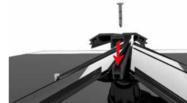
20 Fit the ridge pressure plate by centralising on the ridge and then screwing down using the 4.2 x 45mm screws through the pre-drilled holes.
