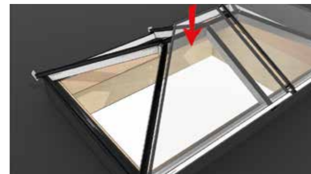
19 Fit glazing around the roof following the roof plan and sit against the lower endcaps. If a roof vent has been specified, follow roof vent installation. Apply pressure to the adhesive of the glazing tape to secure the glass.
