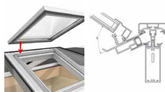
9 Fit vent sash to the vent base by locating the channel in the sash profile into the 2 pivot profiles on either end of the vent base as shown. The sash should be offered at approximately 60° to engage correctly.
